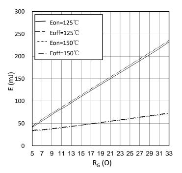
switching losses Diode, Inverter (typical)
